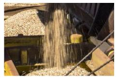
Milling molybdenum, zinc into slowrelease molybdenum fertiliser 11
